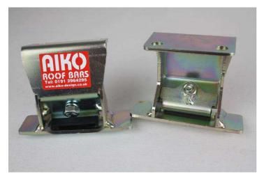
You can probably see how the brackets fit- the lip on the bottom slots under the lip in the van roof, and the little rubber-edged clamp does up with an M8 bolt and spring washer to secure it all in place.
